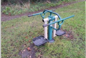
**Finding:** This item has been scaled down and is not covered by the scope of BS EN 16630 which specifically relates to equipment for users of 140cm and above. We have however used our knowledge of this standard to form the basis of our assessment as it is the closest applicable standard available
