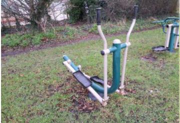
**Finding:** There is/are missing inserts creating finger and the item fails to meet the entrapment from the equipment requirements of BS EN 16630:2015 4.3.6.2 Entrapment of fingers
