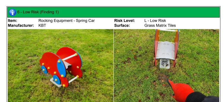
**Finding:** The surface has eroded in some areas and may be **Action:** Reinstate the surface slippery in wet conditions
