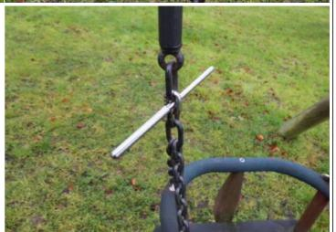
**Finding:** The chain openings are in excess of the 8.6mm as **Action:** Monitor - No action given the risk assessment recommended by BS EN 1176
